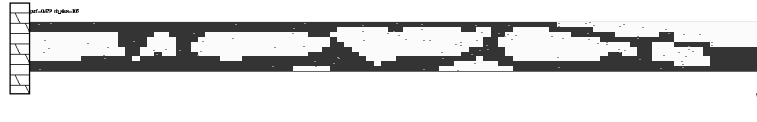
Figure 5.1: Optimal structure on the 100 \times 10 mesh for 10 \times 1 cantilever plate for the Voronoi representation. D_{lim} = 12 , number of cells = 105. weight = 47.9%. CPU time = 14s/gen.
