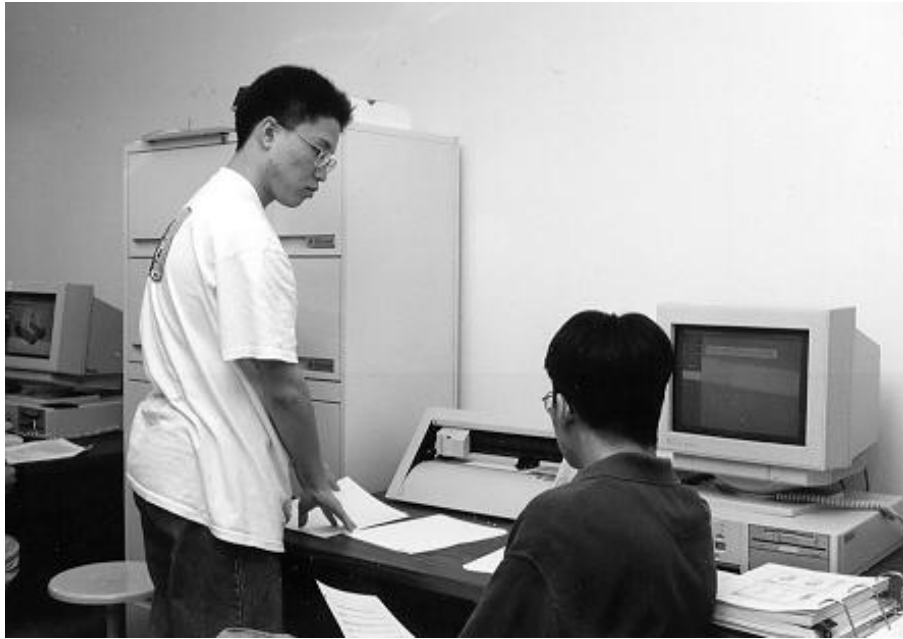
Figure 8: The .STL file is transferred to the JP System 5 prototyping system from Schroff Development Corp. The system cuts the .STL slices of the prototype on sticky paper using a plotter that has a knife blade
