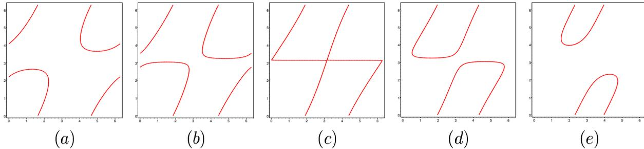
Figure 5: 4-gonal linkage  $\mathcal{P}(1, 3, 1, l_4)$  with  $l_4 \in \{3.5, 3.1, 3, 2.9, 2.2\}$
