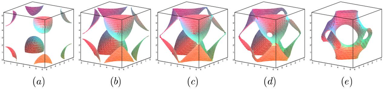
Figure 7: 5-gonal linkage  $\mathcal{P}(1, 1, 1, 1, l_5)$  with  $l_5 \in \{3, 2.1, 2, 1.9, 1\}$
