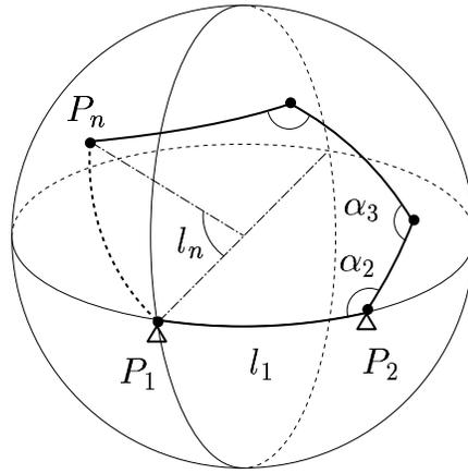
Figure 2:  $n$ -gonal linkage on the unit-sphere
