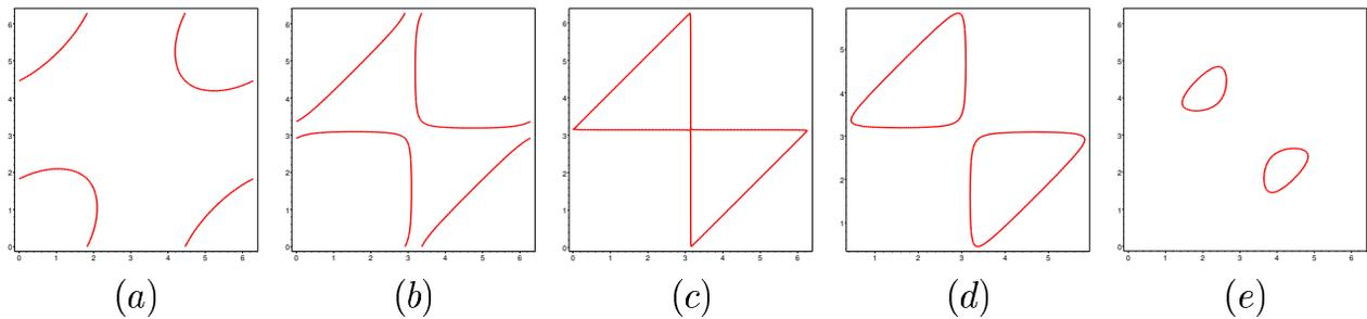
Figure 4: 4-gonal linkage  $\mathcal{P}(1, 1, 1, l_4)$  with  $l_4 \in \{1.5, 1.1, 1, 0.9, 0.5\}$
