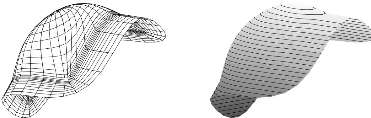
Figure 10: Suitcase corner with user specified closing point and tangent magnitudes
