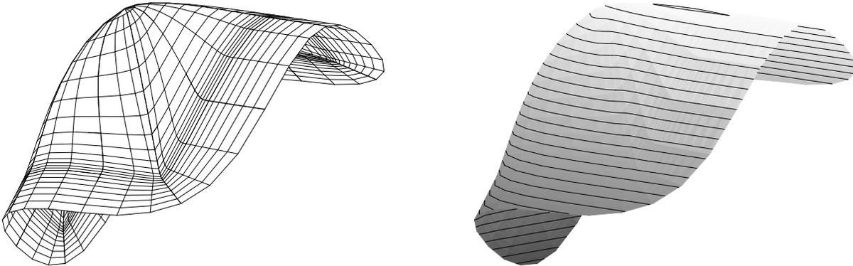
Figure 12: Closing part computed with the extended fairness functional
