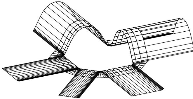
Figure 6: Five-sided hole and the B-spline stripe
