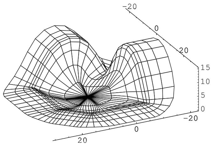
Figure 8: Closing part generated with user specified tangent magnitudes
