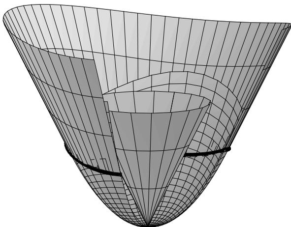
Figure 6: Developable of constant slope as sum of a paraboloid and a cone of revolution.
