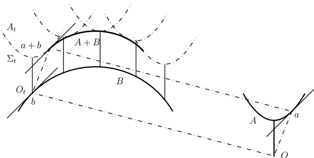
Figure 1: Kinematic generation of the convolution surface
