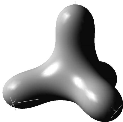
Figure 22: Coastal tetrapod with c^8 = 2.5 a^8 and b = a\sqrt{2}
