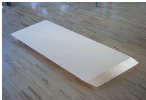
Figure 10: A manufactured panel with an undercut shape
