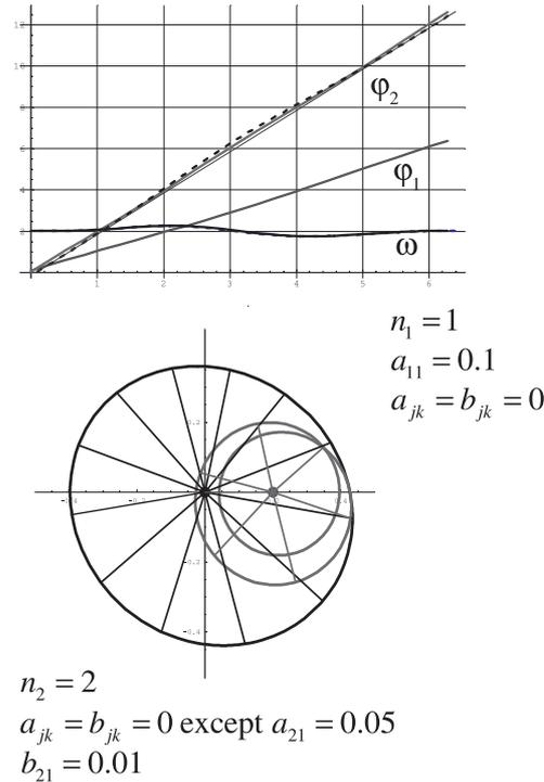
Figure 10: Functions and centrodes of a Fourier ansatz with  $z_1 = 1$ ,  $z_2 = z = 2$
