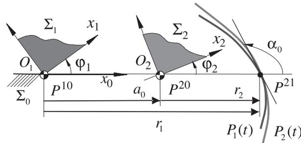
Figure 1: Two planes rotating about two fixed points of a third plane
