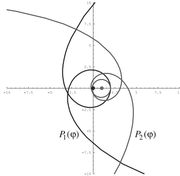
Figure 3: Example centrodes  $P_j(\varphi)$  for the position  $\varphi = 0.1$
