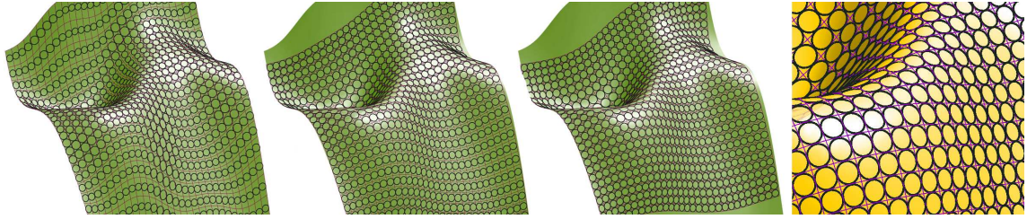
Figure 8: The converging (contracting) grid is perfectly suitable for a circular pattern that covers the surface. Left: Starting position, right (yellowish): converged grid.
