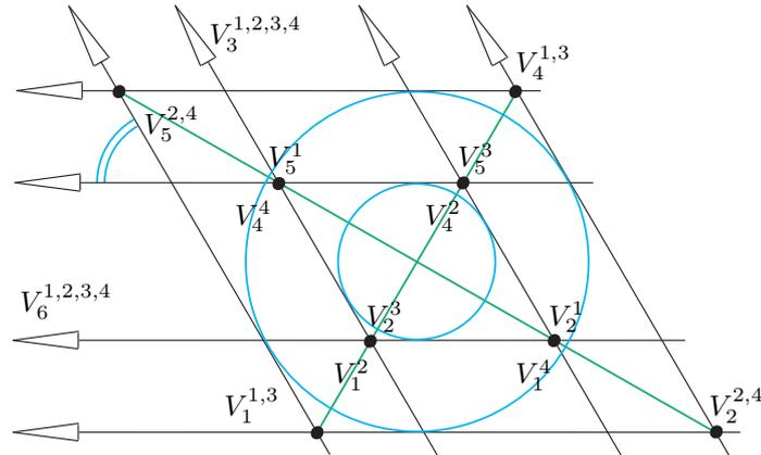
Figure 12: Construction of flexible octahedra of type (III): In the above given construction four flexible octahedra  $V_1^i, \dots, V_6^i$  ( $i = 1, 2, 3, 4$ ) are hidden, where those with indices  $i = 1, 2$  are of type (III): The sides of the three quadrangles spanned by two pairs of opposite vertices touch three concentric circles (which cannot degenerate into the midpoint).
