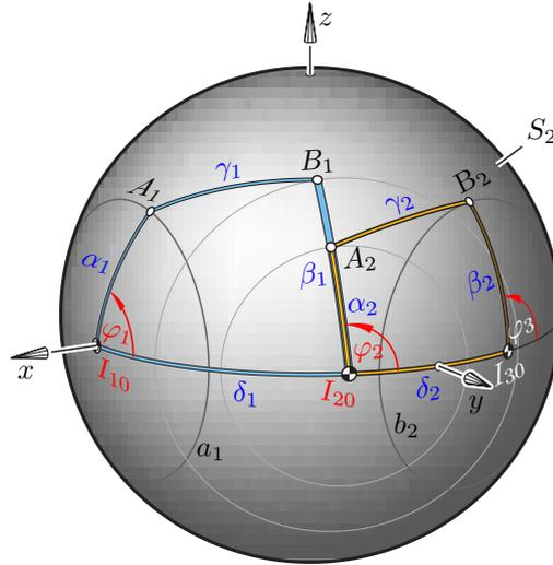
Figure 2: Composition of the two spherical four-bars  $I_{10}A_1B_1I_{20}$  and  $I_{20}A_2B_2I_{30}$  with spherical side lengths  $\alpha_i, \beta_i, \gamma_i, \delta_i, i = 1, 2$  (courtesy H. Stachel)
