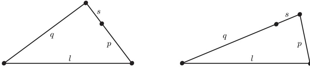
Figure 8: Special poses of the four-bar linkage ( $l = 5, s = 1, p = 2, q = 4$ ) where  $l$  and  $s$  are opposite bars
