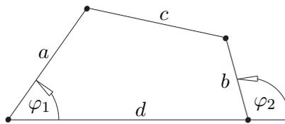
Figure 5: Planar four-bar mechanism with driving arm  $a$ , follower  $b$ , coupler  $c$  and base  $d$
