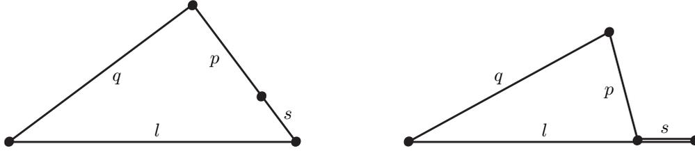
Figure 7: Special poses of the four-bar linkage ( $l = 5, s = 1, p = 2, q = 4$ ) where  $l$  and  $s$  are neighboring bars
