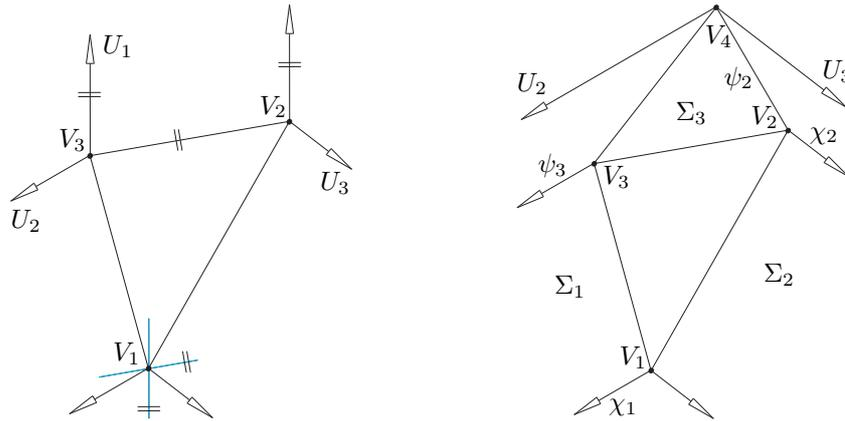
Figure 3: Both figures can be seen as a parallel projection of a spatial structure but on the other hand also as a planar configuration, because such structures has to possess two flat poses.
