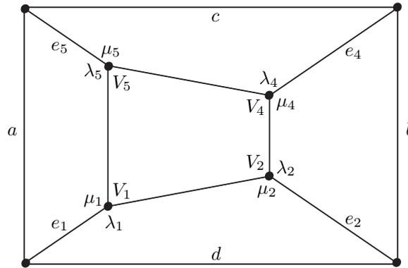
Figure 6: Perspective view of an orthogonal cross section of the prism (= four-bar linkage  $a, b, c, d$ ) and of its four coplanar vertices  $V_1, V_2, V_4, V_5$ . Note that the dihedral angles along the prism edges  $e_i$  are denoted by  $\tau_i$ . Moreover the face angles of the prism at  $V_i$  are denoted by  $\mu_i$  and  $\lambda_i$ , respectively.
