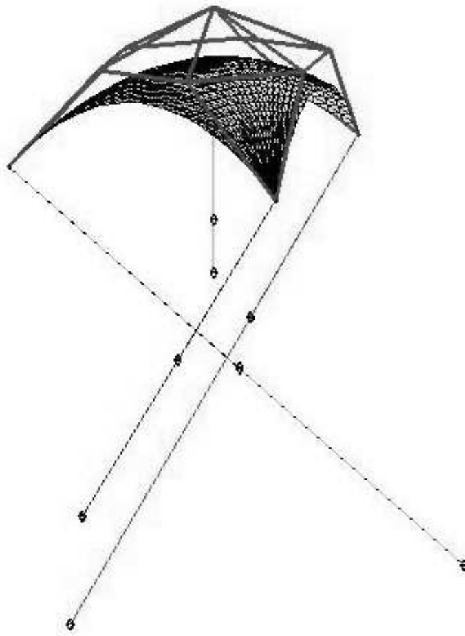
Figure 4: A cubic triangular Bézier patch with normals and their focal points at the corner control points and the “midpoint” P_{111} of the patch.
