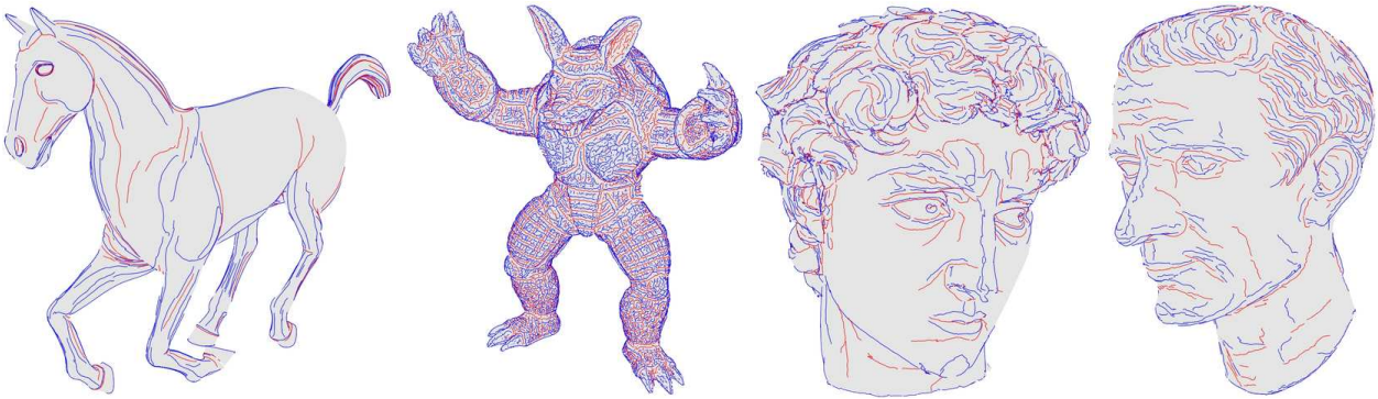
Figure 1: Creases extracted on surface meshes by using the method of [20]. Red and blue lines correspond to the salient extrema of principal curvatures along their curvature lines (a subset of principal direction ridges called crest lines), respectively.
