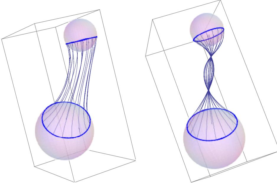
Figure 7: Curvatures not satisfying the restrictions at the endpoints of the spine curve may yield self-intersections of the resulting surface (right). Smooth blending surface can be obtained for the same initial data with an appropriate choice of spine curve (left).
