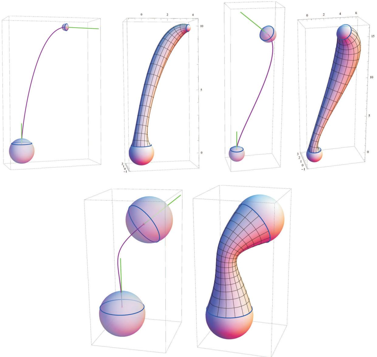
Figure 6: Three positions of initial data, each with the spine curve (left) and the computed surface (right).
