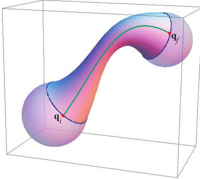
Figure 2: A surface blending the given spheres touching them at the given circles.
