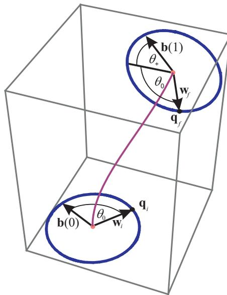
Figure 4: The rotation-minimizing map  $q_i \rightarrow q_f$  between the perpendicular unit circles at the end points of the curve  $\boldsymbol{\alpha}(t)$ .
