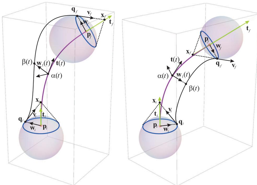
Figure 5: Visualization of various notations in two different positions of initial data (with unit spheres). The spine curve  $\alpha(t)$  (purple) and one of the parameter curves  $\beta(t)$  (black) can also be seen.
