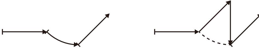
Figure 7: A general path having an arc element (left) can be converted to LGP (right) by replacing the arc with two connected line elements
