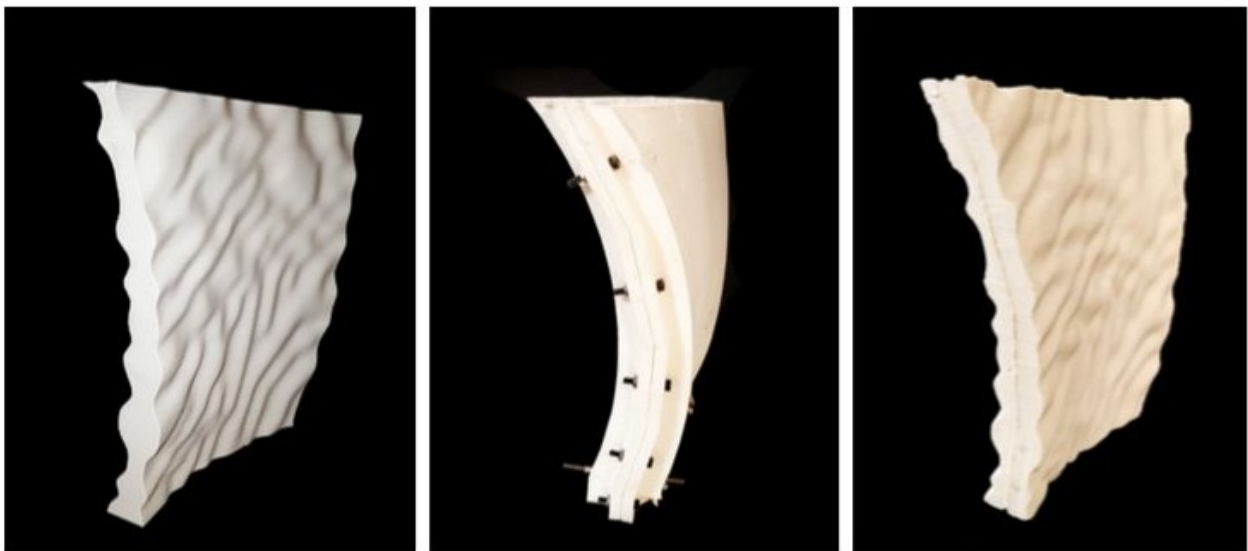
Figure 9: 3D-printed parts of the tessellation shell. (Project by Anja KUNIC, Aleksandra ROCHALA, Mateusz REJNIAK)
