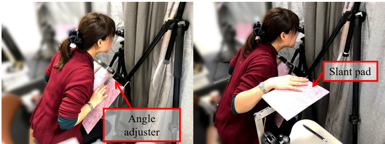
Figure 7: Photos from the experiment. Left: the participant was using an angle adjuster to report the perspective angle. Right: the participant was using a slant pad to report the optical slant angle.
