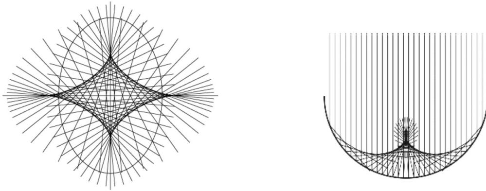
Figure 2: Two examples of caustics: the evolute of an ellipse as an envelope of the set of normal rays (left) and one often used for amplification of signals in parabolic satellite dishes (right).
