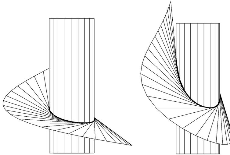
Figure 4: Frontal projections of the torses with a reverse edge on a cylinder, constructed according to parametric Equations (13): a)  $a = 0.3$ ; b)  $a = 0.6$ ; c)  $a = 0.9$
