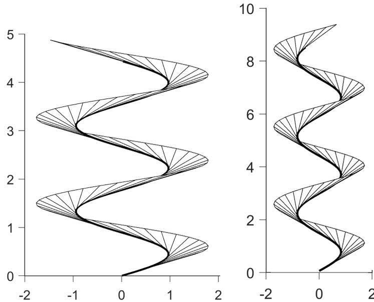
Figure 2: Frontal projections of the torsos of helicoids bending on each other by changing the angle of ascent of the reverse edge: a) angle of ascent  $\beta = 17^\circ$ ; b) angle of ascent  $\beta = 34^\circ$ .
