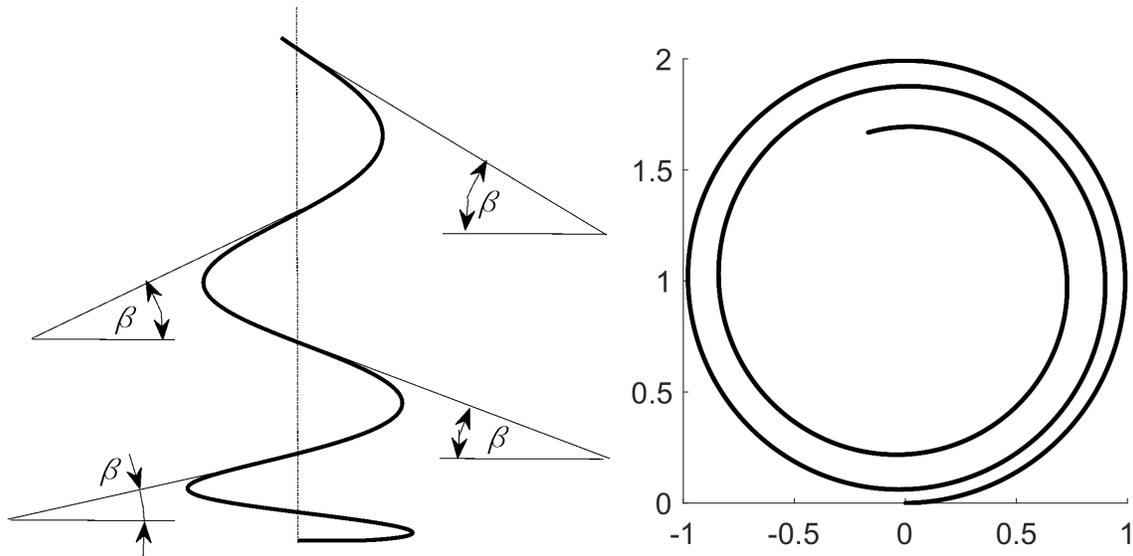
Figure 1: Projections of a constant curvature curve with a linear law of increasing the angle of ascent: a) frontal projection; b) horizontal projection.
