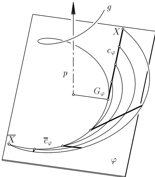
Figure 6: Shade and shadow lines in  $\varphi$
