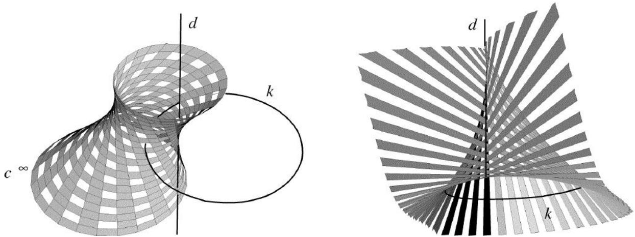
Figure 4: The conic  $c^\infty$  is determined by a one-sheet hyperboloid which contains the line  $d$  as a generator. The pedal surface is the conoid of  $3^{rd}$  degree with the nodal line  $d$  and it contains the circle  $k$  and the conic  $c^\infty$ .
