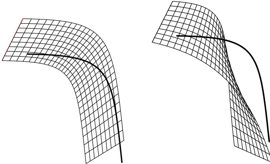
Figure 7: Ruled surfaces, generated by the rational approximation to the rotation minimizing frame (left) and by the Frenet–Serret frame (right).
