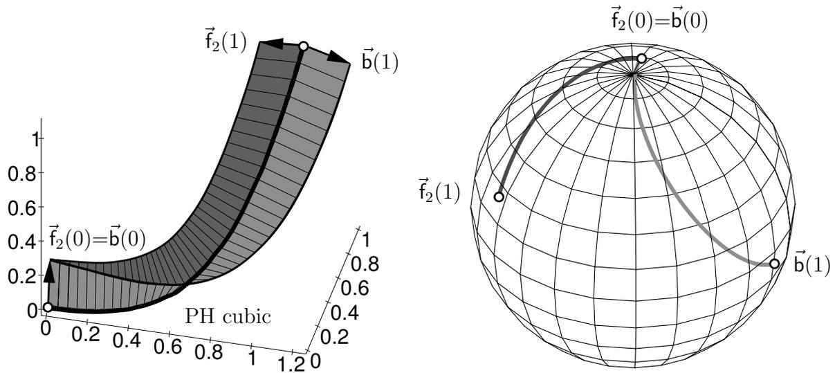
Figure 5: Rotation minimizing frame vs. Frenet-Serret frame of a PH cubic. The vector fields  $\vec{f}_2(v)$  and  $\vec{b}(v)$  along with the PH cubic (left), and the associated spherical indicatrices  $\vec{f}_2(v)$  and  $\vec{b}(v)$  (right)
