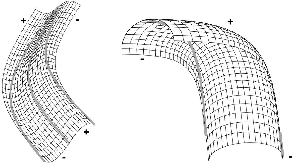
Figure 2: Parabolic lines on profile surfaces and signs of the Gaussian curvatures.
