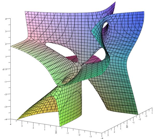
Figure 12: Singularity surface of spherical 3-RPR manipulator
