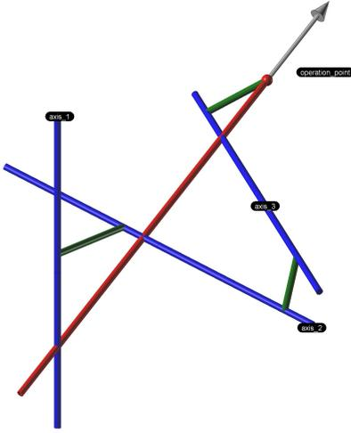
Figure 5: Singular position of the operation point
