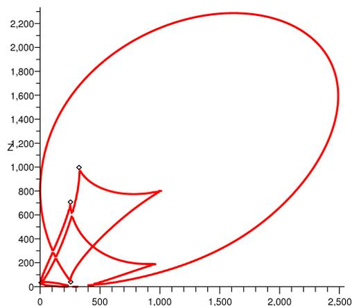
Figure 14: Horizontal cross-section of the singularity surface in joint space
