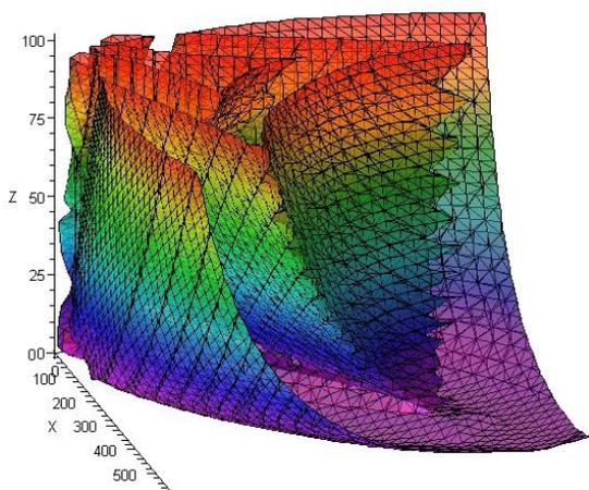
Figure 13: Singularity surface of a planar 3-RPR manipulator in joint space
