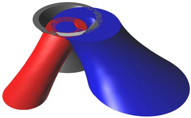
Figure 8: Workspace of a 3-RPR manipulator
