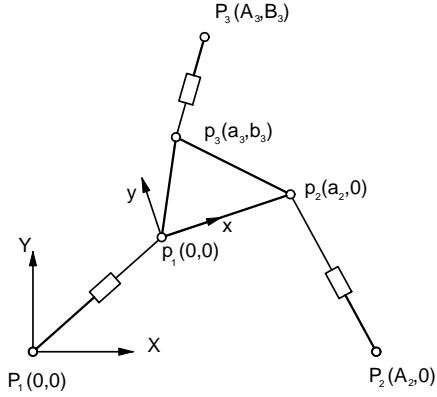
Figure 7: Planar 3-RPR parallel manipulator
