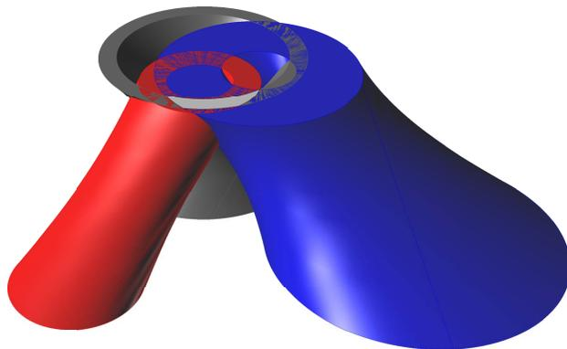
Figure 8: Workspace of a 3-RPR manipulator
