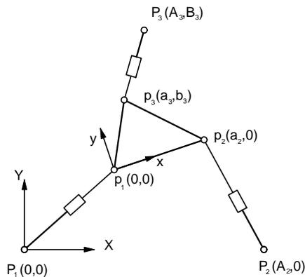
Figure 7: Planar 3-RPR parallel manipulator
