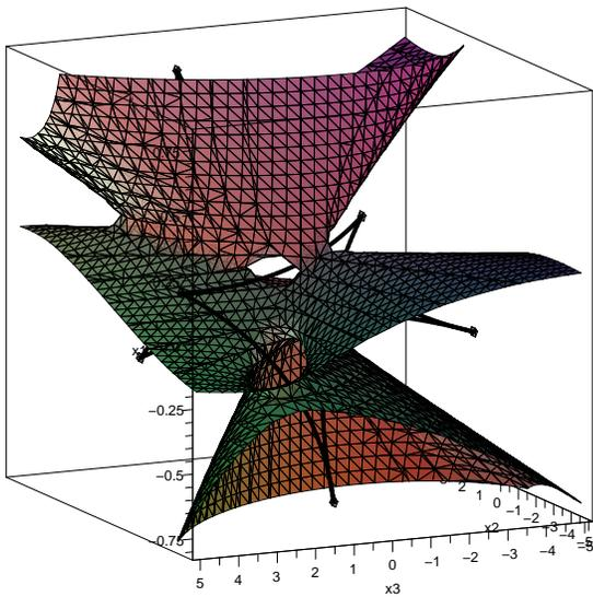
Figure 11: Singularity surface of a planar 3-RPR manipulator in kinematic image space
