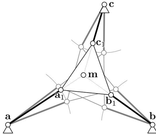
Figure 10: Singular pose of a planar 3-RPR manipulator
