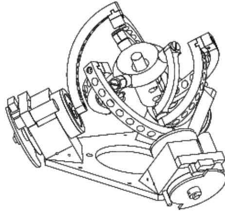
Figure 16: CAD model of *The Agile Eye* (courtesy Prof. C. GOSSELIN)
